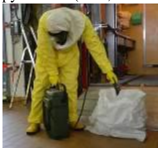
Identification of an unknown sample by hand-held GC-MS apparatus in a potentially hot zone
