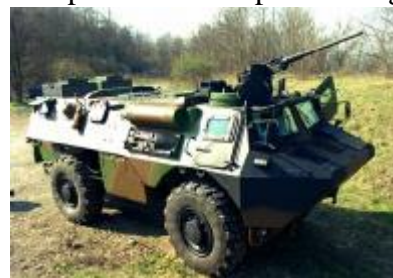
Military-oriented reconnaissance armoured VBR NBC vehicle equipped with detection and identification instruments for chemical, biological and radiological hazardous agents
