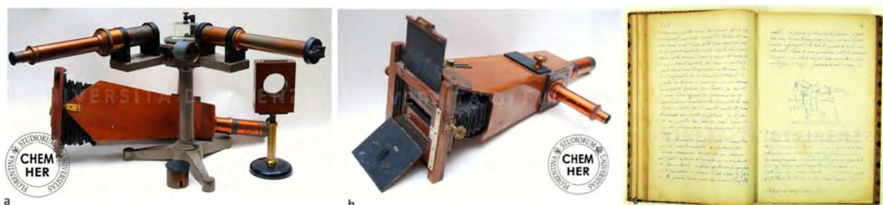
Figure 3. The spectroscope used for the didactics experiments (a), its photographic chamber (b) and Ugo Schiff lecture notes, in which it is described (c)
