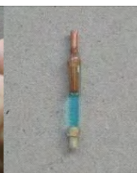
Figure (4) Prepared copper /copper sulfate electrode with no air bubbles
