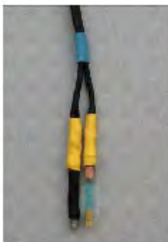
Figure (15) Finished Sb and Cu/CuSO 4 electrodes
