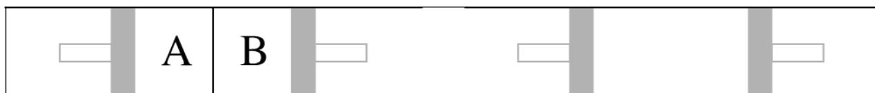
Figure 1 - Left: hydrogen (A) and chlorine (B) are separated by a diaphragm; Right: the same system after removing the diaphragm.
