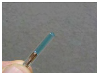
Figure (2) Solution should be filled to the top of the small tubing. Slight excess as judged by an almost overflow.
