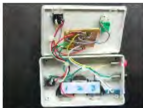
Figure (8) Exposed interior of utility box (three 3V lithium button-type batteries are labeled as 1, 2 and 3)
