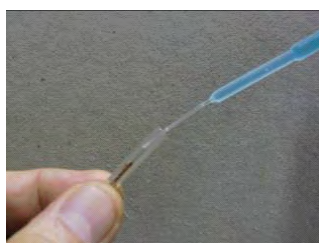
Figure (1) Use a micro-tip plastic pipette to fill the small compartment with 1M \text{CuSO}_4 solution
