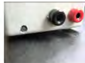
Figure (10) Small side opening for adjusting set correction 1K \Omega trimmer pot
